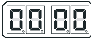
Figure 10-11: Display Station A/D’s No Station Transfer Button Depressed
